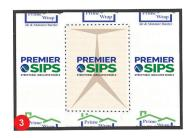
Make and inverted Y cut in the at rough opening. Then cut straight across the top and make diagonal cuts from the top corners to create header flap.
