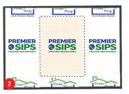
Continue to unroll the Building Wrap tightly around the structure - covering all door and window openings. While nailing or stapling make sure the fabric is taut against the exterior wall and not sagging. Seal all seams, tears, and cuts with Building Wrap Sheathing Tape.
