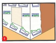
Start with lowest course, 2-3 feet from a corner. Secure Building Wrap firmly in place by fastening it every 12" to 18" along the vertical studs using large-headed or plastic cap nail or 1" crown staples.
