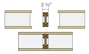
TYPE L SPLINE: Double 2x dimensional lumber spline, having a width of 3".
