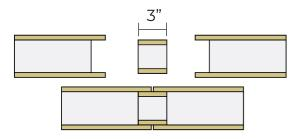
TYPE I SPLINE: I-Joist spline, having a width of 2 1/2".
