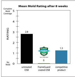
Independent testing by Forintek Canada Corporation, using ASTM D-3273. Project 4528
