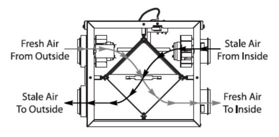
This cross-flow unit is rated at around 60%, depending on temperature and pressure
